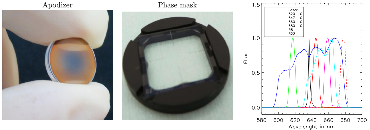
Figure 7. Left: Apodizer used with DZPM. Middle: DZPM phase mask. Right: Spectra used in our experiment.
